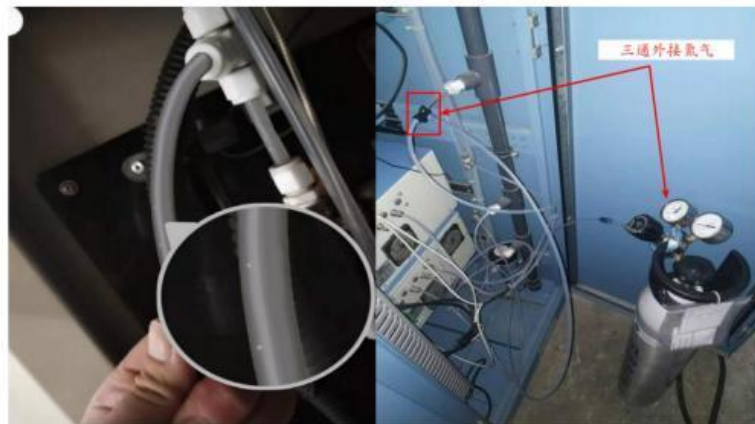
进样管路被人为钻孔示例图，进样管路接三通被稀释示例图
