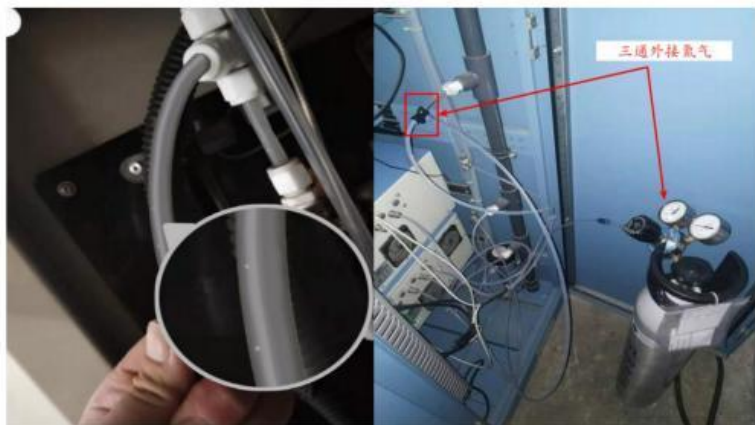
进样管路被人为钻孔示例图，进样管路接三通被稀释示例图
